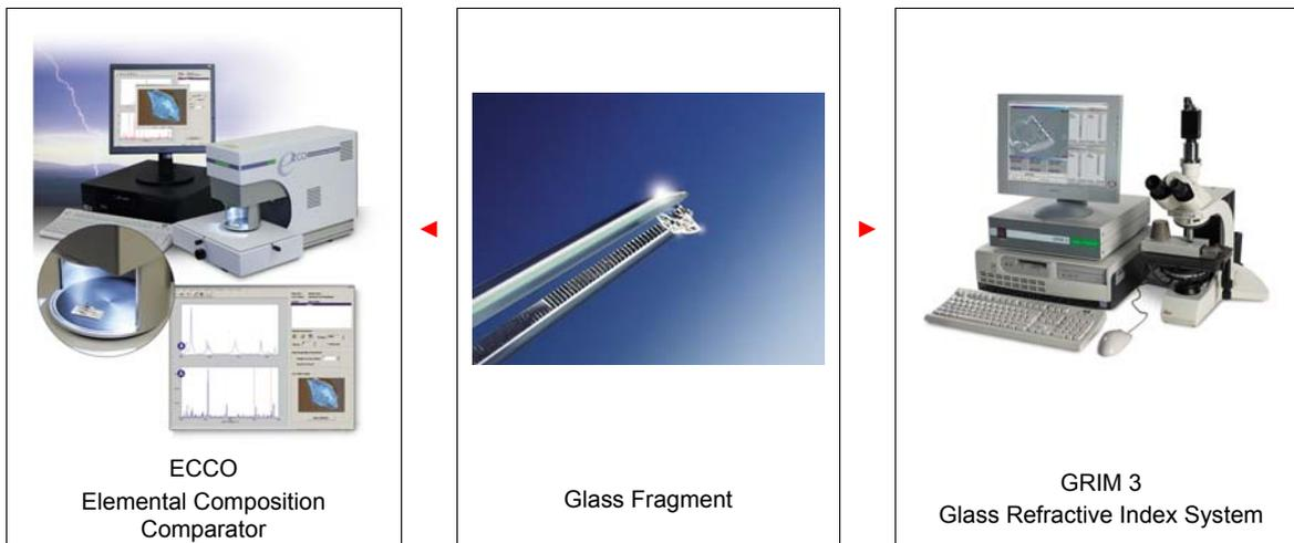
One of the most widely applied techniques for the forensic analysis of glass involves the measurement of its refractive index (RI) using the oil immersion method. The Foster + Freeman Glass Refractive Index Measurement (GRIM) system is a compact and convenient instrument intended for this purpose.
